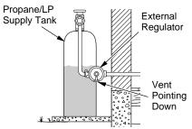
Figure 14 - External Regulator With Vent Pointing Down
